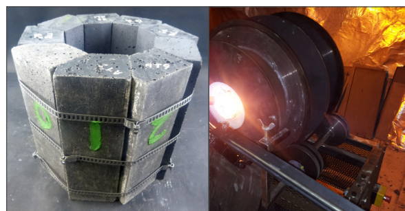
Figure 8 Rotary Slag Testing Configuration
