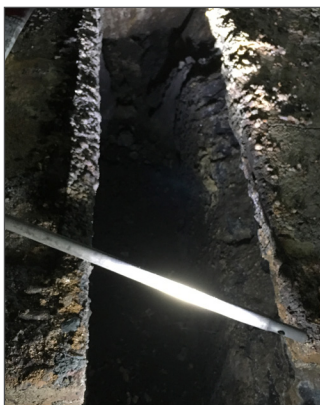
Figure 12 Slag Separator after 12-day campaign
